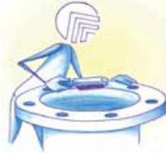
Examine the flange surfaces, fasteners (bolts or studs), nuts and washers to ensure they do not have any serious defects. Replace any components if found to be defective. If in doubt, seek advice from a qualified expert.
