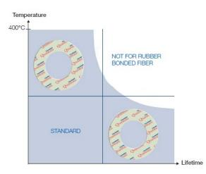
Fibrous rubber-bonded gaskets harden when exposed to heat - some more quickly than others. The effects of thermal cycling (especially in steam applications) can often lead to flanged assembly failures. A more flexible gasket with superior compressibility and recovery properties will withstand greater pressure and temperature fluctuations resulting in a more reliable joint.
