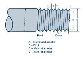
In the above figure, the arrows point to the root and the crest of the threads. The pitch of the thread is the distance from the crest of one thread to the crest of the next thread. This measurement is used to determine the number of threads per inch, or millimeters per thread, data that are usually supplied by the fastener manufacturer. The one most frequently used term in designating the size of a bolt or screw fastener is its nominal diameter.
